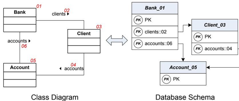
Figure 1: A class diagram and corresponding database schemata
