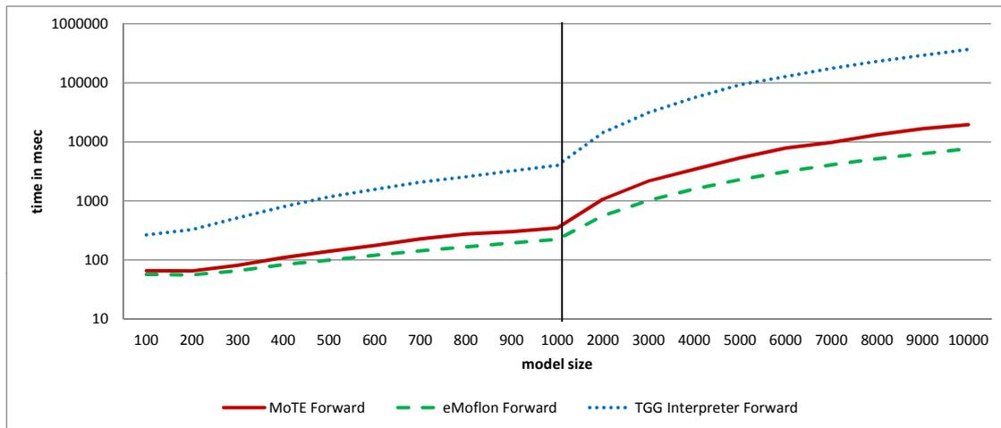
Figure 7: Runtime Measurement Results for Forward Transformation
