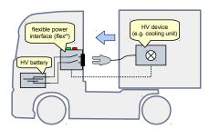
Figure 1:  $flex^{Pi}$  connects a cooling trailer to a hybrid truck
